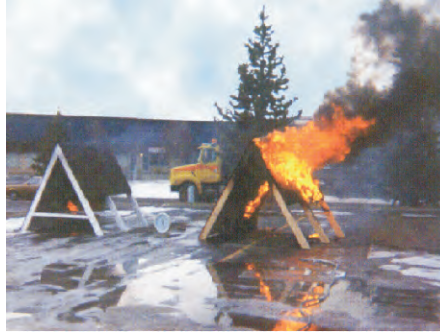
SafeCoat coated interior roof space and an untreated roof space under identical fire conditions
